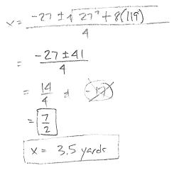
32. A tunnel, with a parabolic arch, is 8 mtrs wide. If the height of the arch 1 mtr from the outer edge of the arch is 3mtrs, can a truck that is 6 mtrs tall and 3 mtrs wide fit through the arch? Draw and label a diagram. Determine an equation that models the arch of the tunnel. Support your answer with the appropriate calculations. If you determine the truck is too tall, determine what truck width would support the height.
